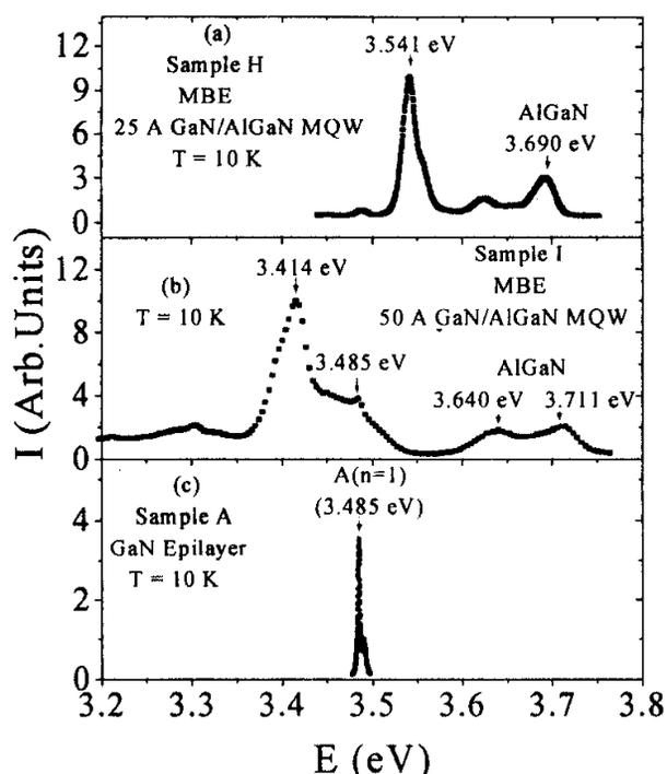
Fig.3. PL emission spectra of GaN/AlGa<sub>1-x</sub>N MQWs (a) and (b), and GaN epilayer (c) measured at  $T = 10$  K.
