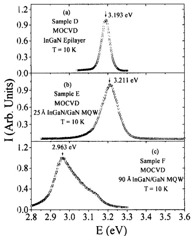
Fig. 2. PL emission spectra of In<sub>x</sub>Ga<sub>1-x</sub>N/GaN MQWs (b) and (c), and In<sub>x</sub>Ga<sub>1-x</sub>N epilayer (a) measured at  $T=10$  K.
