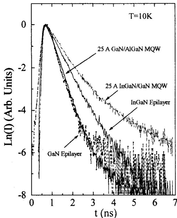
Fig. 4. PL temporal responses measured at the spectral peak positions for MBE and MOCVD samples: GaN and In<sub>x</sub>Ga<sub>1-x</sub>N epilayers, GaN/AlGa<sub>1-x</sub>N and In<sub>x</sub>Ga<sub>1-x</sub>N/GaN MQWs.
